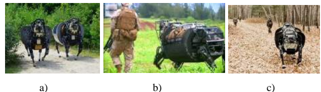
Fig. 1. Boston Dynamics robot mules: a) Carrying heavy loads; b) Following soldiers; c) Moving through complex terrains
